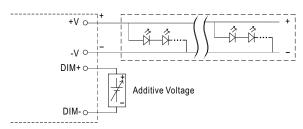
"DO NOT connect "DIM- to -V"
