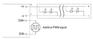
"DO NOT connect "DIM- to -V"
